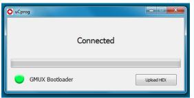
Press the **Upload HEX button** to select the firmware file to upgrade. Pressing Ok the firmware writing procedure on the GMUX microcontroller starts and the leds blink alternatively. On the display of G801 - G802 module appear the progressives of the number of packets transmitted and received during the procedure. The bar on the software window shows the progress of the procedure.
